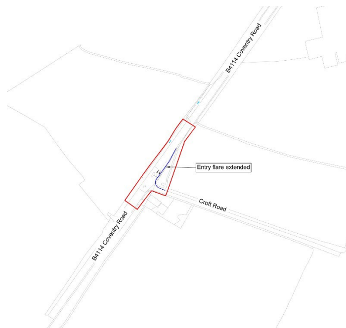
Fig 54. Proposed Works to Coventry Road / Croft Road junction east of Croft (Document Reference 6.3.3.3)
